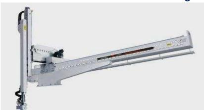
BRTN Series is applicable to all types of horizontal injection machine ranges of 650~4000T for take-out products and sprues. Three-axis driven by AC servo motor, take-out at super high-speed (1.5sec.). Easy for E-O-A-T adjustment, long using life and low failure rate, applicable to take-out products with short forming cycle or complex automatic, such as auto products, washing machine and household appliance products take-out.
